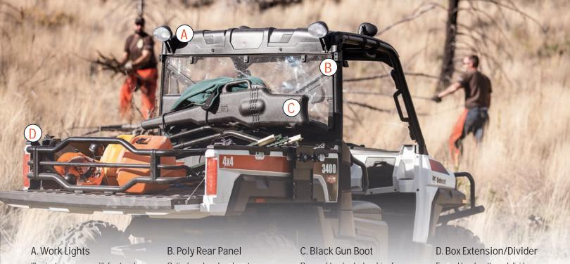
Illuminate your area with front and rear work lights. Lights can be mounted to cab frame, poly roof, or steel roof. Front and rear require front power leads P/N 7229408 or 7260989 and 7260991 for gas.
